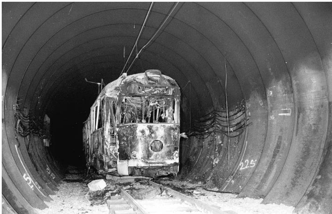
Fig. 3: test fire in a subway tunnel under realistic conditions
